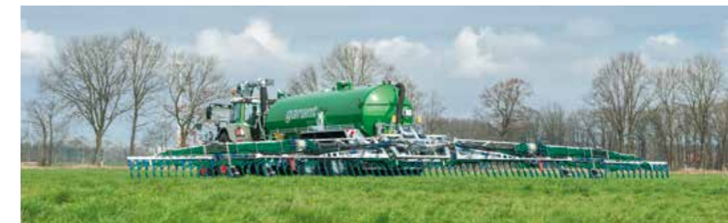
BOMECH trailing shoe distributor Multi 21 m
