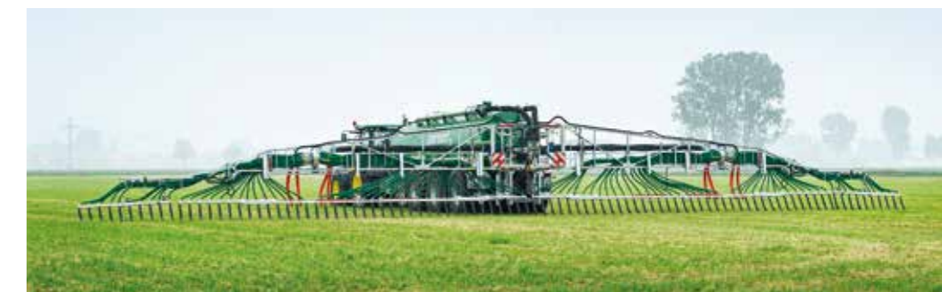
Vogelsang trailing shoe distributor SwingMax Slide 30 m
