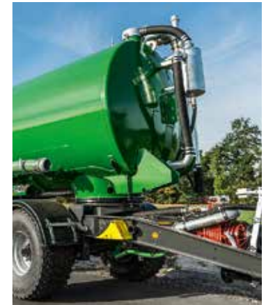
Mechanically driven compressor with rotary union
