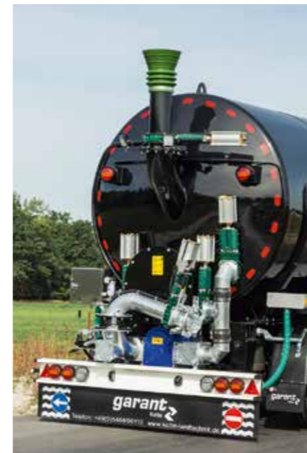
Docking funnel at the top of the container rear wall (TSA)
