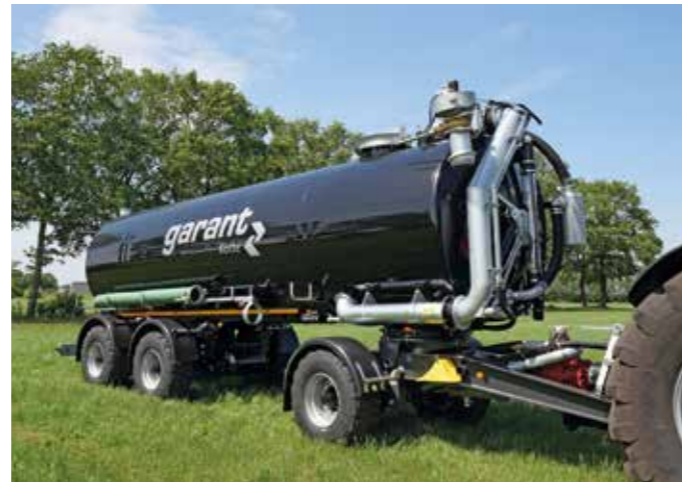
TAV with suction arm with two swivel joints and one filling dome
