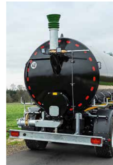
Docking funnel at the top of the container rear wall (TAV)
