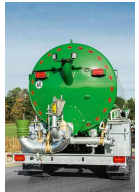
Docking funnel at the bottom of the container rear wall (TAV)
