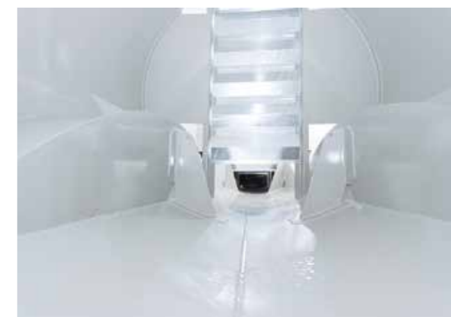
Bolted baffles and Sika Permacor internal coating
