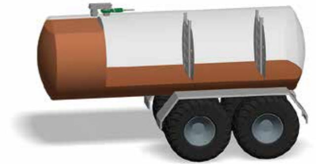
Baffles in the two-chamber system
