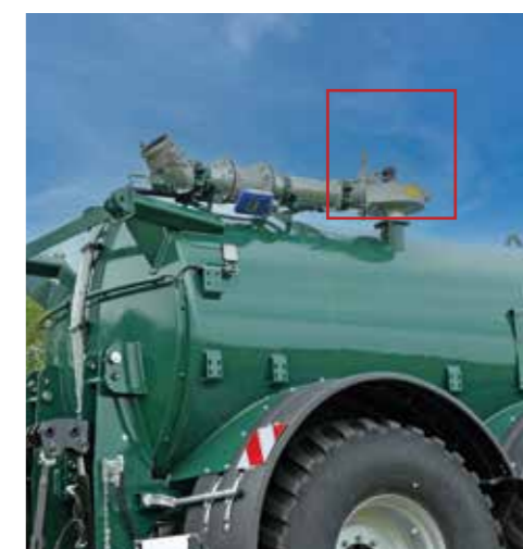
Pressure accelerator on the vacuum barrel
