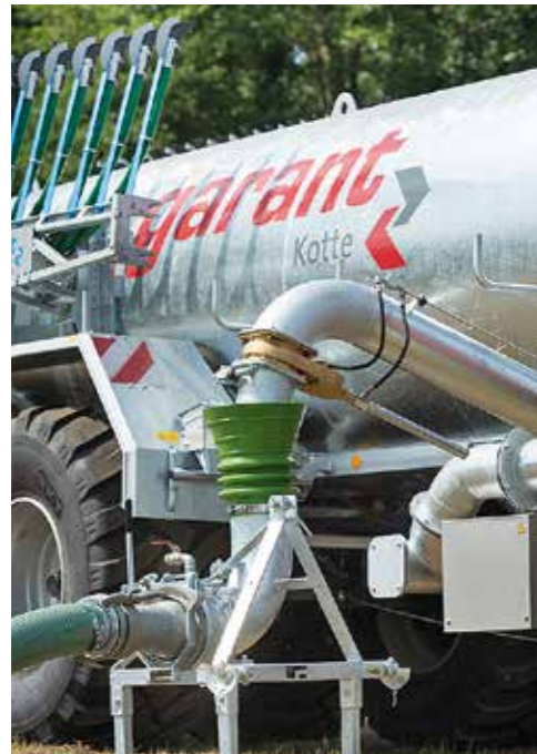
Docking station for pits
