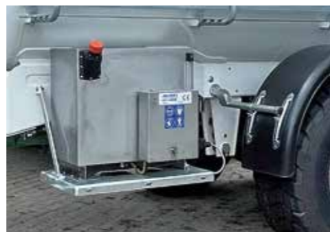
Dosing system for nitrification inhibitors
