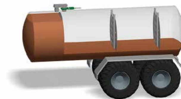
Baffles in the two-chamber system
