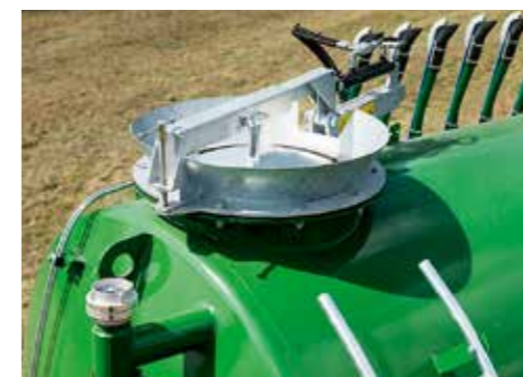
Hydraulic filling dome with hinged lid for vacuum tankers
