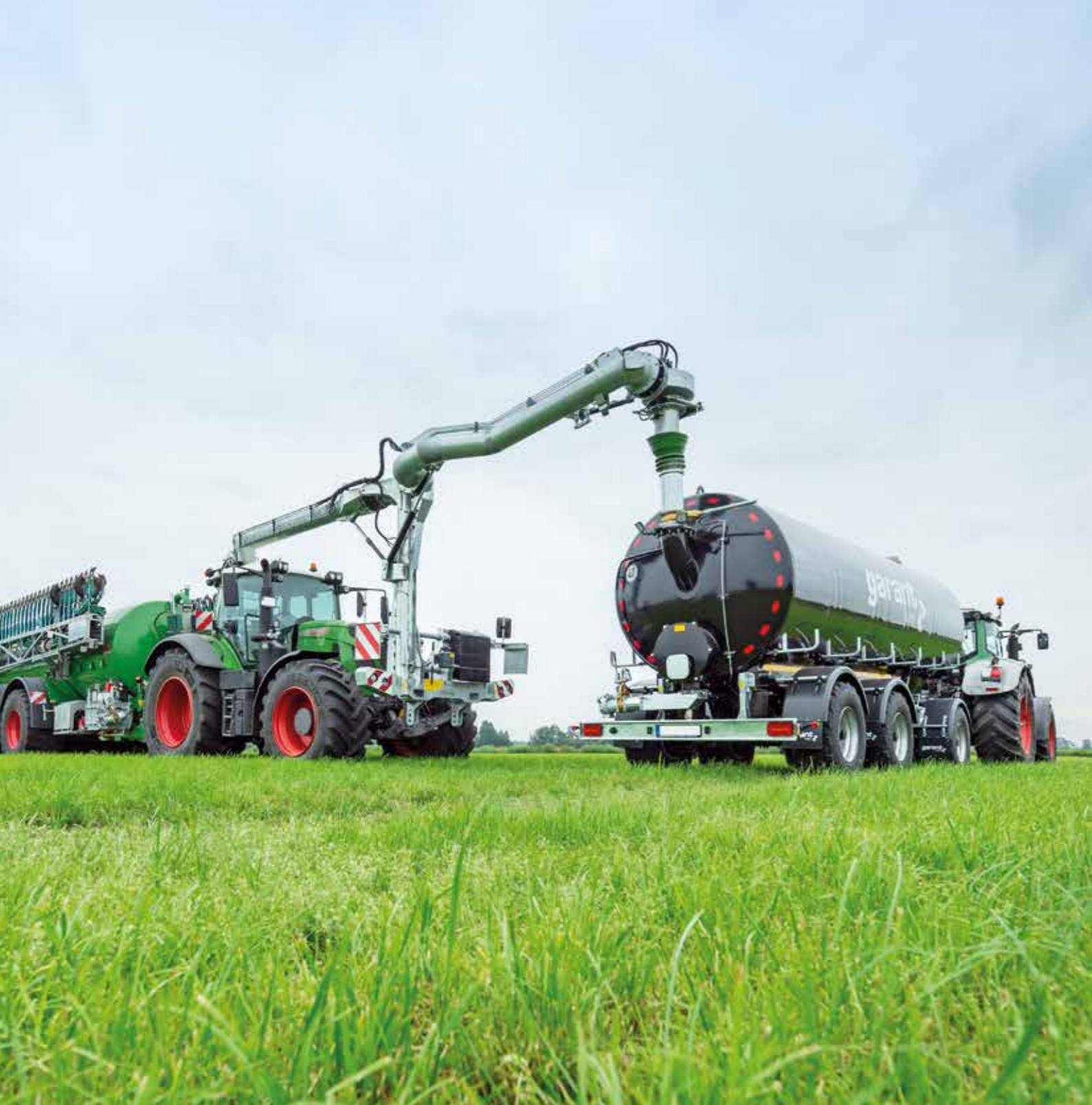
Suction arm with a swivel joint
