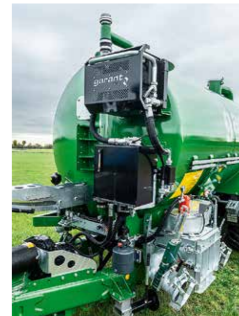
Pump tanker with on-board hydraulics
