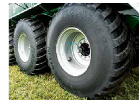
PTG Tyre pressure control system with two-pipe system
