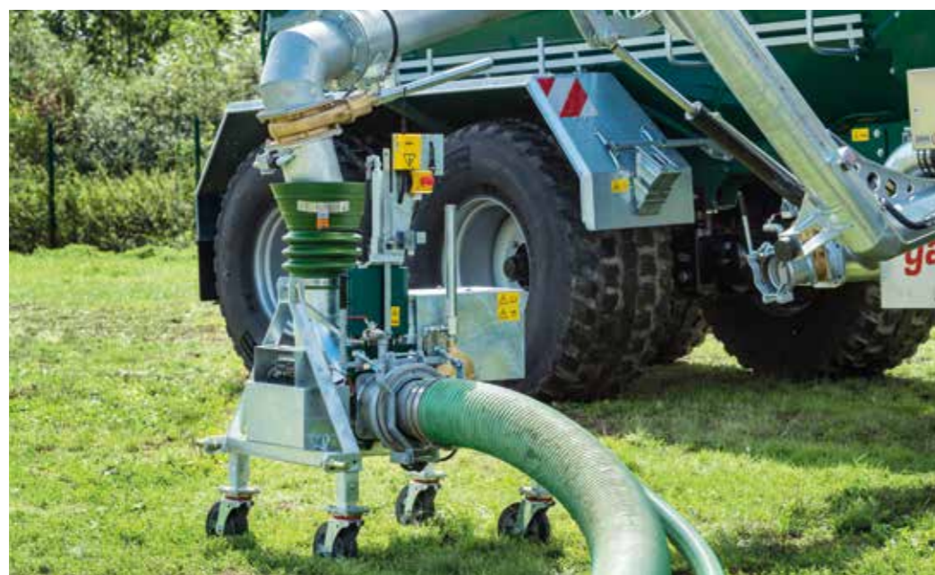
Radio docking station for elevated tanks and pits
