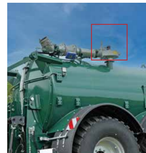
Pressure accelerator on the vacuum barrel
