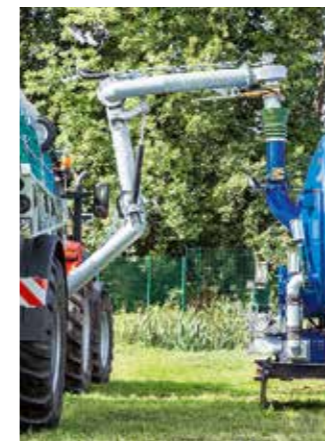
Suction arm with two swivel joints
