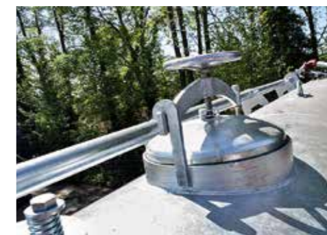
Mechanical filling dome with swivel lid for vacuum tankers
