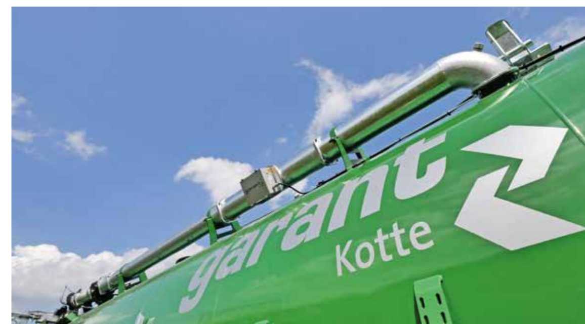
NIR sensor on pump tanker
