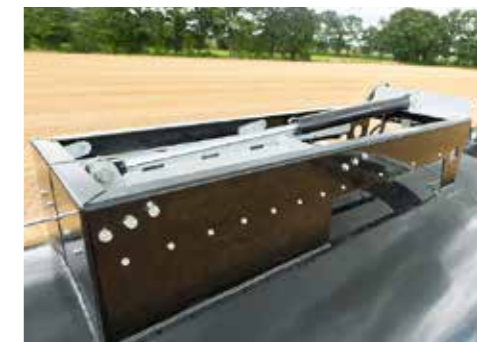
Hydraulic filling dome with sliding lid for pump tankers
