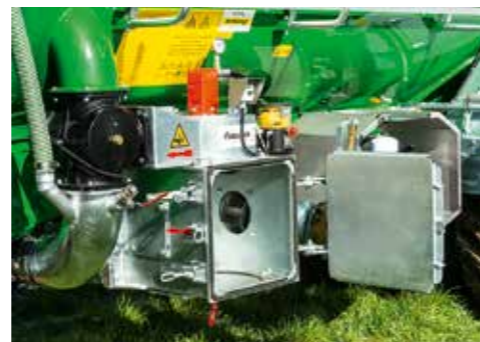
Cutterbar device with stone trap
