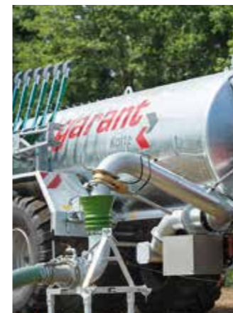
Suction arm with a swivel joint
